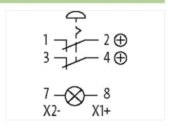
PIN 1: N/C 1 Male PIN 2: N/C1 PIN 3: N/C 2 PIN 4: N/C 2 PIN 5: n.c. PIN 6: n.c. PIN 7: (X2/-) PIN 8: (X1/+)
