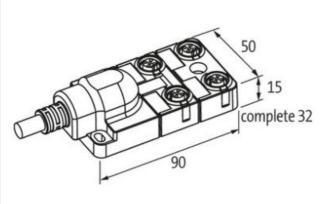
5 (PE 4 (N/O)-(ST) 3(-) 2 (N/C) - (S2) 1441 ye/bn rd/bu white n/ye rowr lue i/pk greet pa n.c. n.c. free arrangeable, contact 1:1 on terminals for 4 signals per port, PIN5 bridged on terminals
